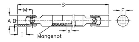
$A = 40 \\ F = 20 \\ Longitudinal ribs = 6x21x25 \\ M = 54 \\ MD max N m = 80 \\ s = 301 \\ T = 32 \\ x = 40$
